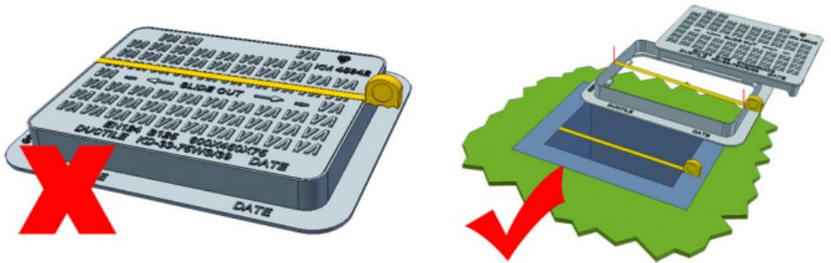
Many customers will measure the 'visible' or 'lid' size of the cover which is larger than the clear opening (hole size) often stating 650x550mm or 25"x18" (inches) these usually all have a 600x450mm clear opening dimension. Manhole covers must be larger than the clear opening (hole) to prevent them falling into the chamber.
